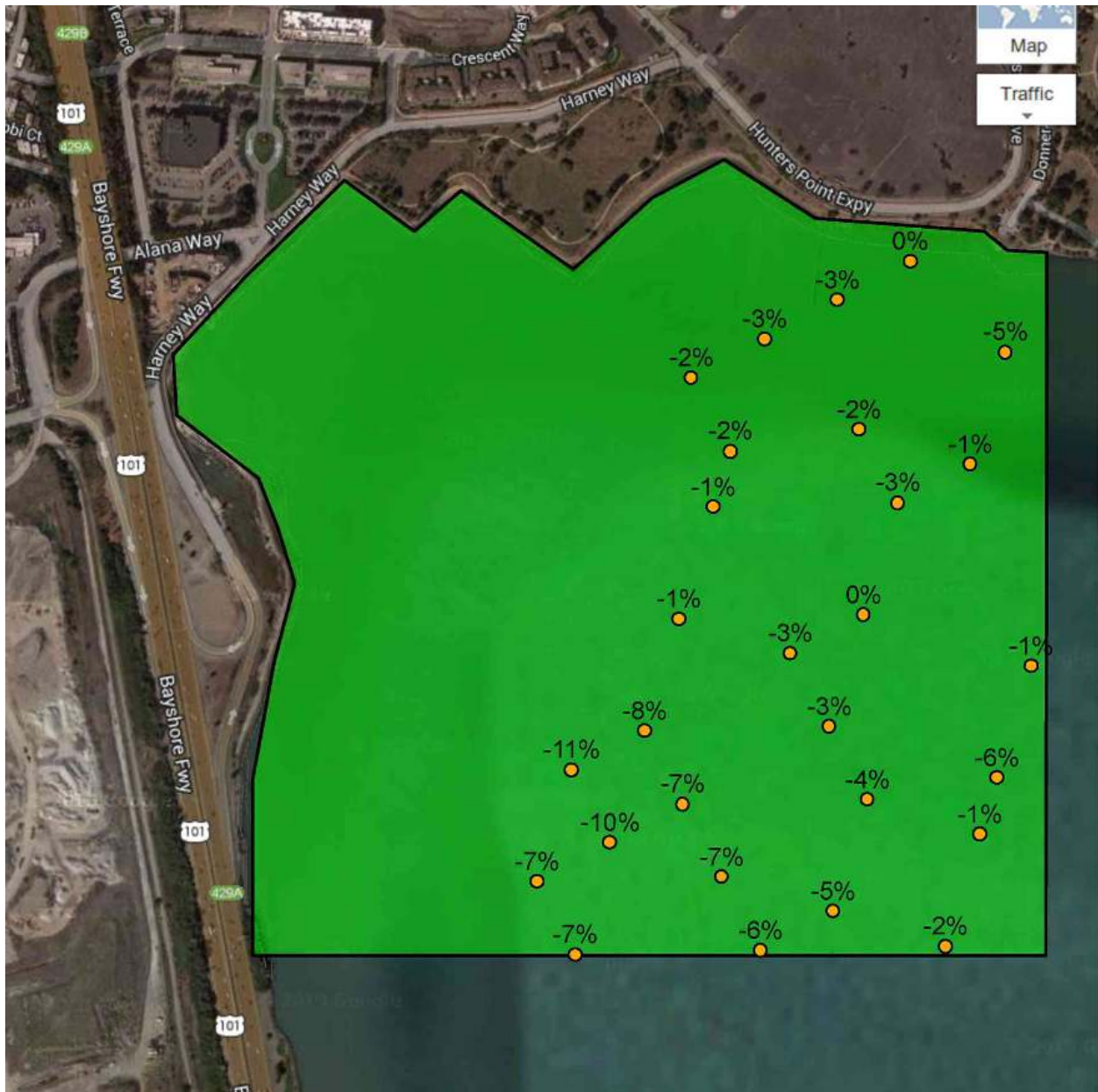
Figure 7: Data points collected from the 2012 wind tunnel study for the West wind direction. Near-shore areas are not examined.
